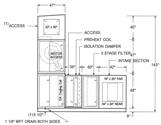
(1) Addes access doors to discharge plenum, added dimension to drain elevation.
